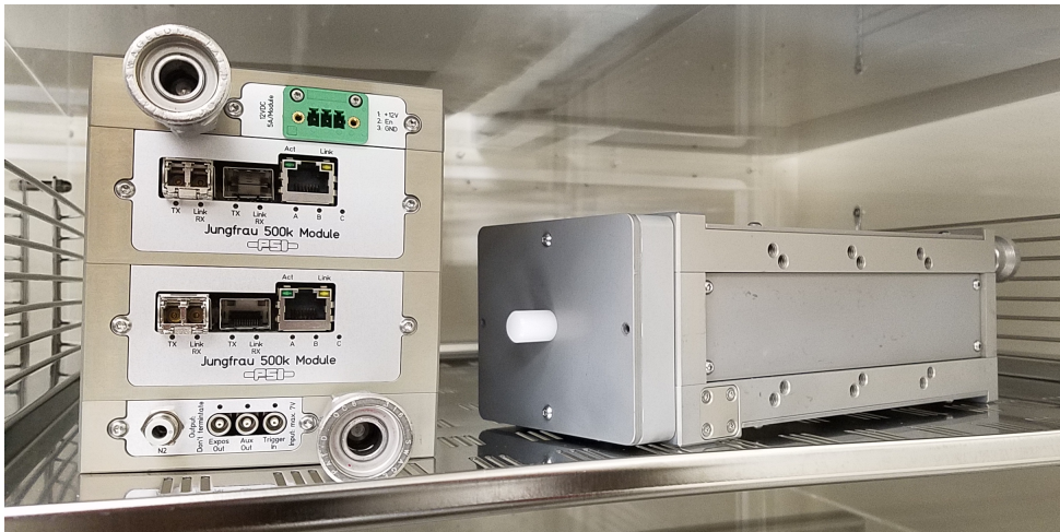
On the left, 1M camera from back. On the right, 0.5M camera with cover in place.
