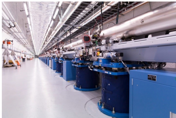
The 100-meter-long undulator: where the coherent x-ray photons are born.
