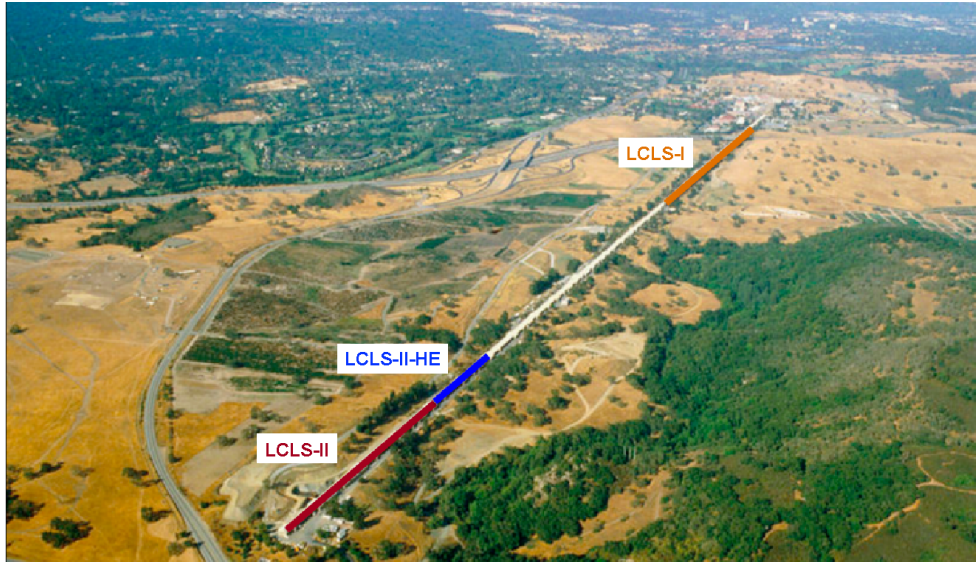
Figure 5 Layout of the accelerator upgrades for LCLS-II and LCLS-II-HE in relation to the existing linac (LCLS-I). The SLAC site and Stanford campus can be seen in the upper right.
